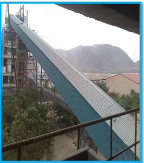
Covered belt conveyers provide for the control of fugitive dust emission
